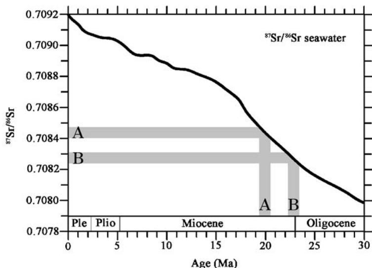
Fig. 2. Curve of seawater strontium isotopic composition for the last 30 Ma, after McArthur and Howarth (2004).  $^{86}\text{Sr}/^{87}\text{Sr}$  data for samples A and B were measured by the methods described in Table 1.
